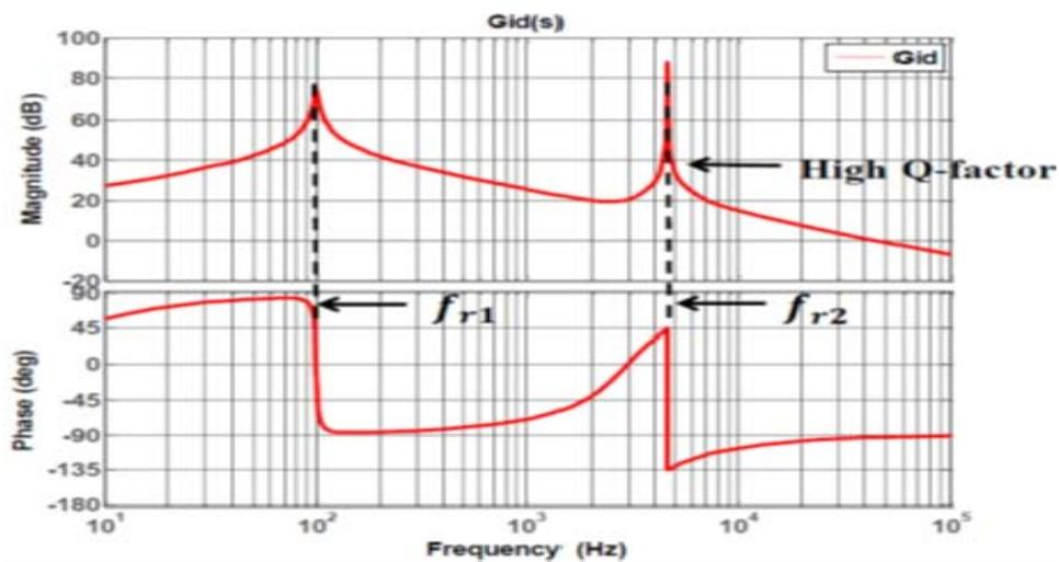
Figure 2. Frequency response of input voltage
