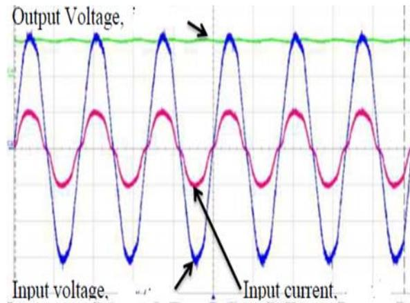
Figure 12. Input AC and output DC signals of proposed converter
