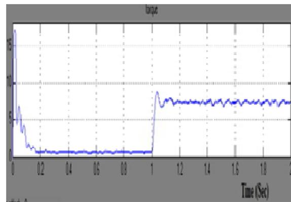
Figure 8. Change in load torque at time  $t= 1$  sec
